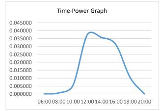
A graph plotted for power generation in watts against time in open ground
