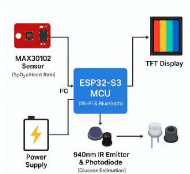
Fig. 4. Block Diagram of Non-Invasive Blood Glucose Monitor
