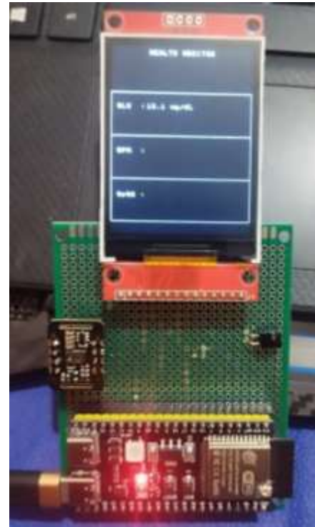
Fig .2. The mounting of the sensors and the ESP32-S3
