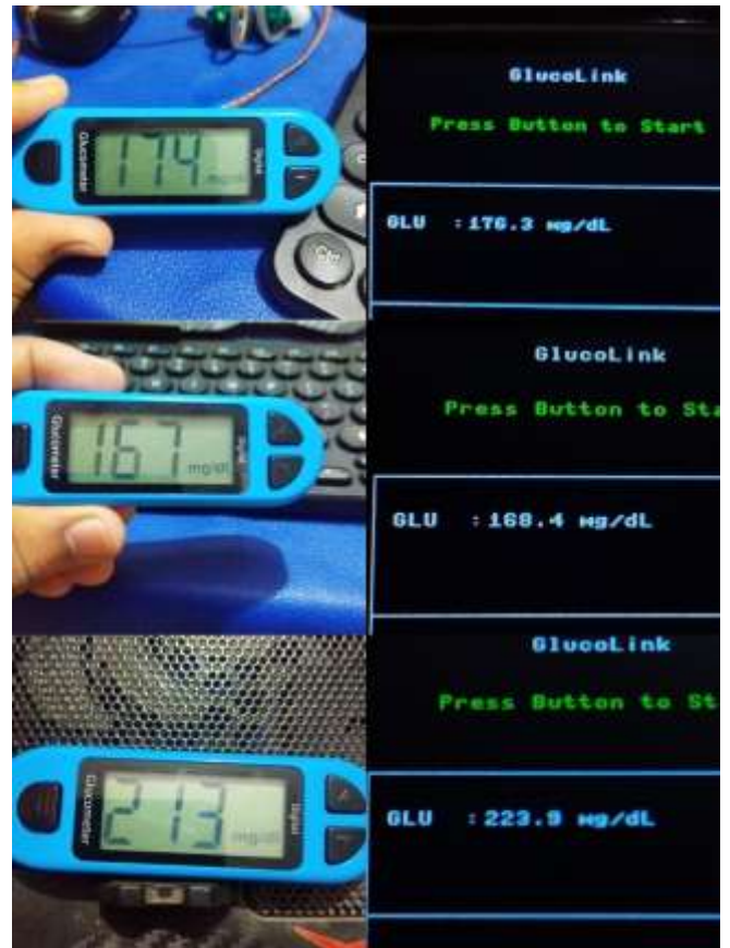
Fig.7. Comparison between our Non-Invasive Blood Glucose monitor and Invasive Blood Glucose Monitor
