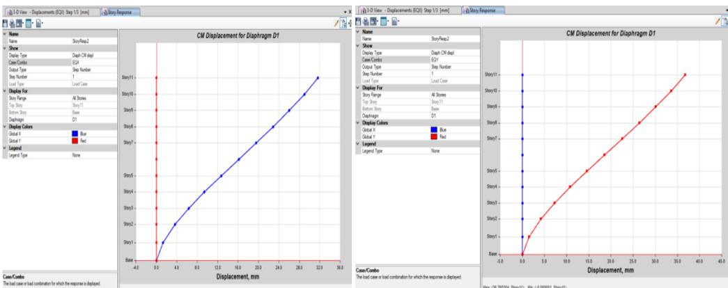
**Figure 8 Diaphragm CM displacement in EQ X & Y**
