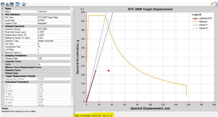
b) **Figure 15 a) Performance point for PushX for model1 b)Performance point for PushX for model2**
