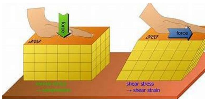
Figure 2 Force deformation characteristics.
