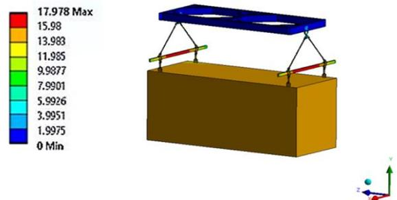
Figure 24 Total deformation at 100% loading
