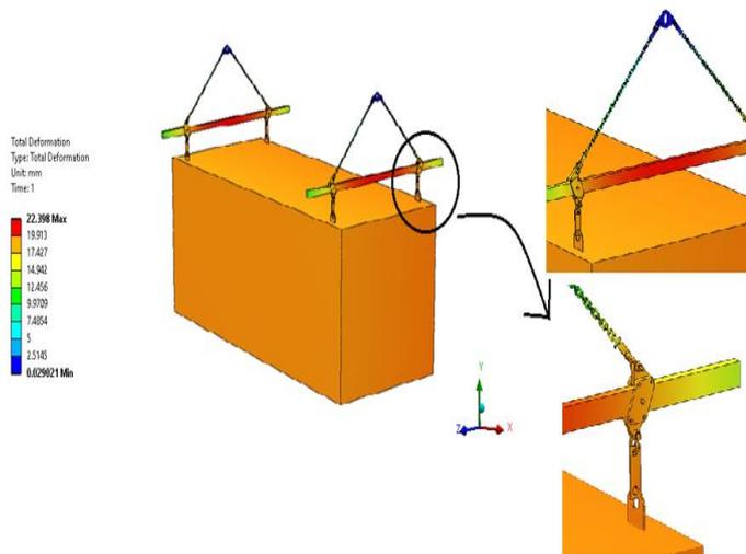
Figure 12 Total deformation of MSMS
