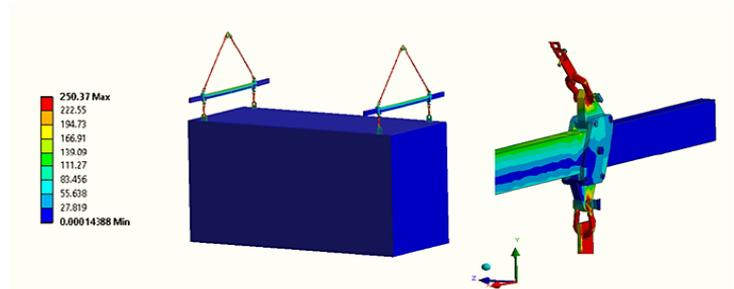
Figure 17 Equivalent stress of MSMS at 40°C
