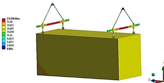
Figure 16 Total deformation of MSMS at 40°C
