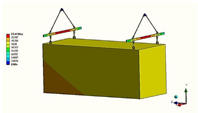
Figure 18 Total deformation of MSMS at 50°C
