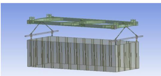
Figure 3 Container with slings and multiple spreader bar attachment
