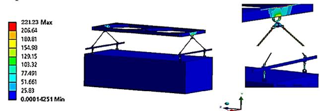
Figure 25 Equivalent stress at 100% loading
