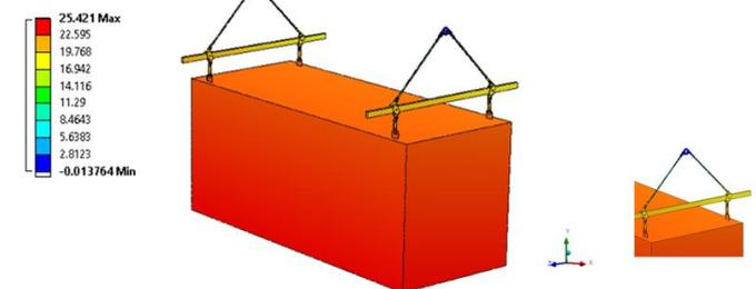
Figure 14 Total deformation of MSMS under inertial load
