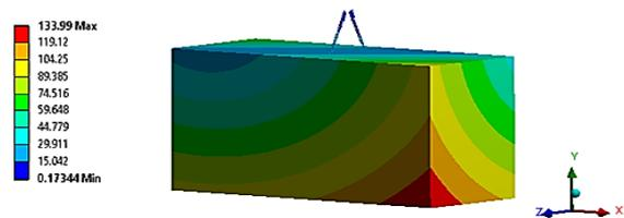
Figure 5 Total deformation of MS
