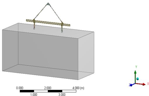
Figure 2 Container with two sling and spreader attachment
