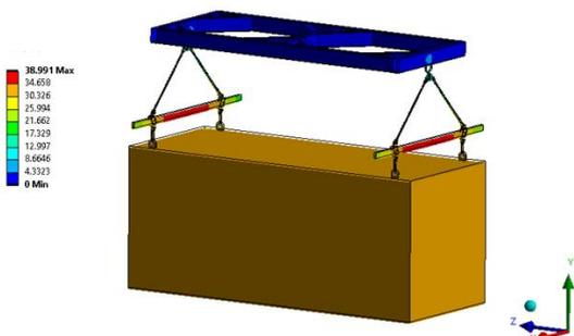
Figure 28 Total deformation at 150% loading
