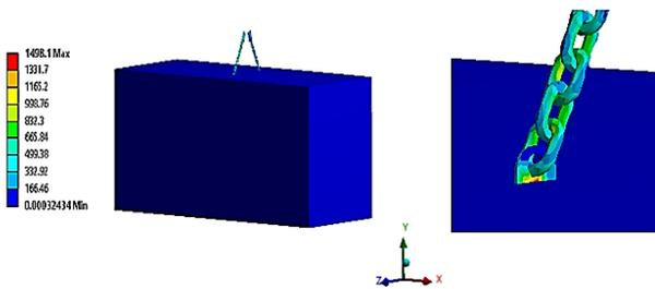
Figure 7 Equivalent stress of MS
