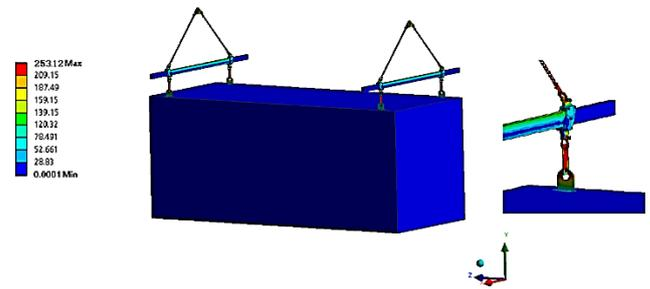
Figure 19 Equivalent stress of MSMS at 50°C
