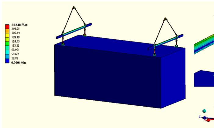
Figure 21 Equivalent stress of MSMS at 50°C
