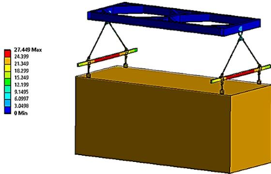
Figure 26 Total deformation at 120% loading
