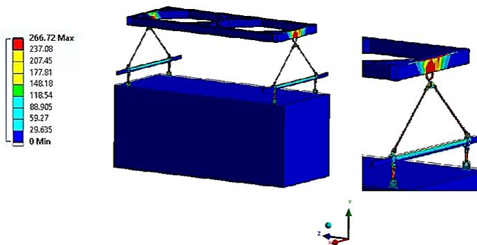
Figure 27 Equivalent stress at 120% loading
