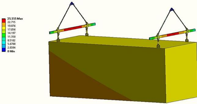
Figure 20 Total deformation of MSMS at 60°C
