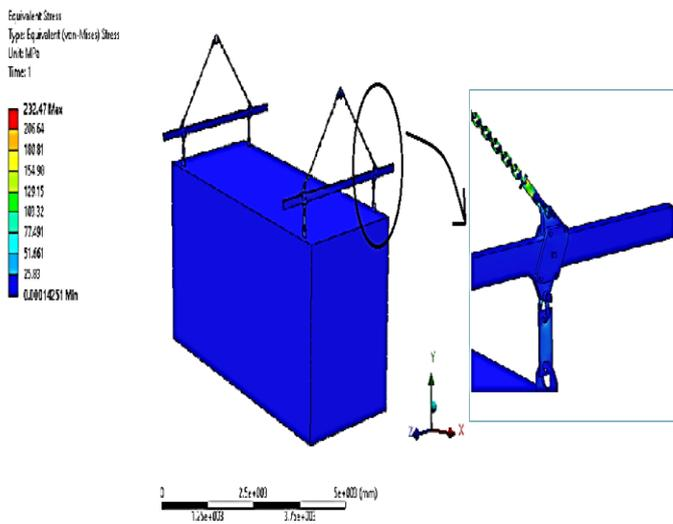
Figure 15 Equivalent stress of MSMS under inertial load
