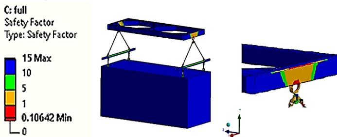
Figure 22 Safety factor of whole structure
