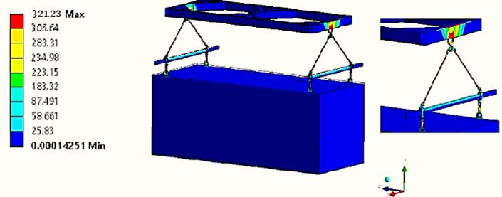
Figure 29 Total deformation at 100% loading
