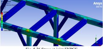
Fig. 5.26 Stress at joint FYPGF
