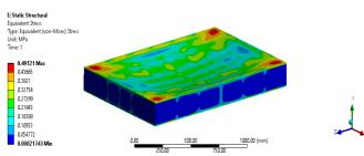
Fig. 5.10 Equivalent stress of GYC95
