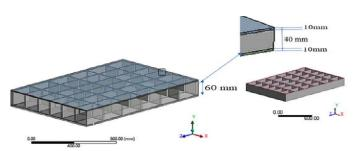
Fig. 5.20 Model of Wooden Panel of Yellow Poplar with Polyethylene (10 mm /40 mm/10 mm) (WYP60)
