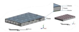
Fig. 4.4 Grid type panel of Yellow Poplar with CFRP (GYC95)
