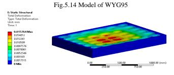
Fig. 5.15 Total deformation of WYG95
