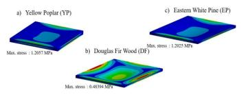
Fig. 5.3 Equivalent stress of various wooden panels (CLT)
