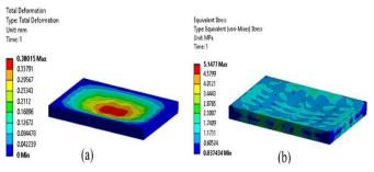
Fig. 5.5 WP70: (a) Total deformation (b) Equivalent stress
