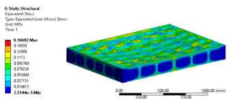
Fig. 5.13 Equivalent stress of GYC95
