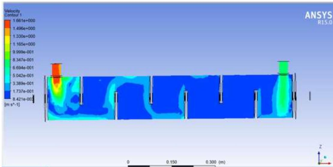
Fig 4.1: Velocity counter obtained in Ansys Fluent Post processing for Model with 20% baffle cut
