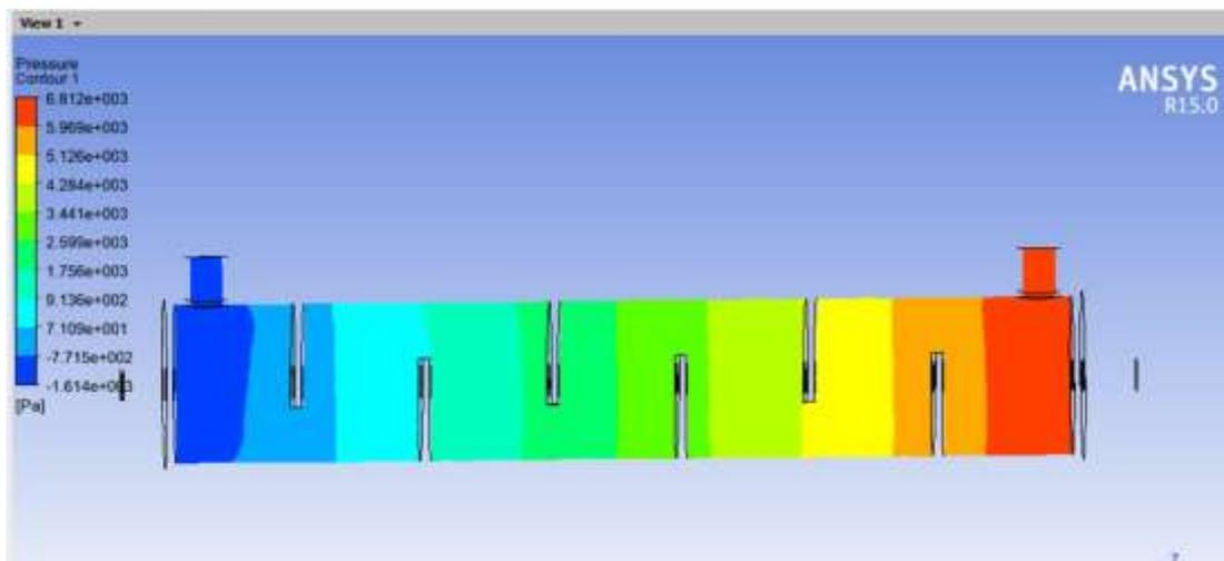
Fig 4.1: Pressure counter obtained in Ansys Fluent Post processing for Model with 20% baffle cut
