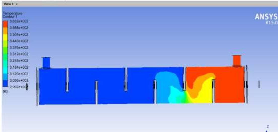
Fig 4.3: Temperature counter obtained in Ansys Fluent Post processing for Model with 20% baffle cut
