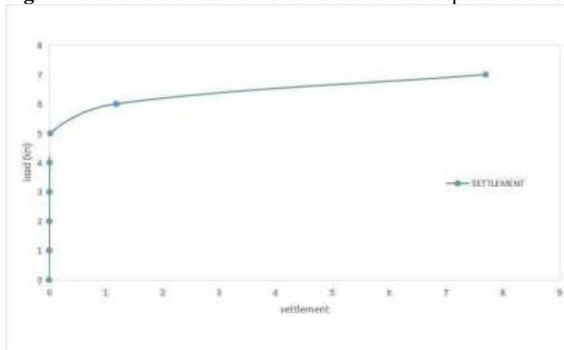
**Fig. 2** Reaction force versus vertical displacement in Abaqus
