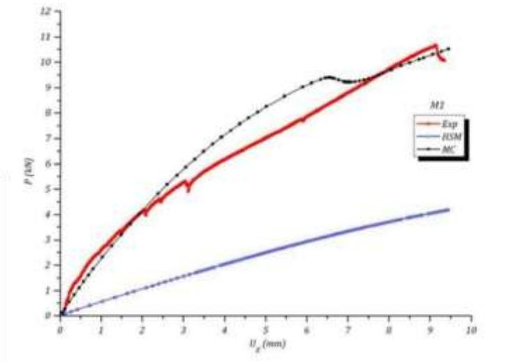
**Fig. 1** Evolution of the reaction force versus vertical displacement from reference paper.
