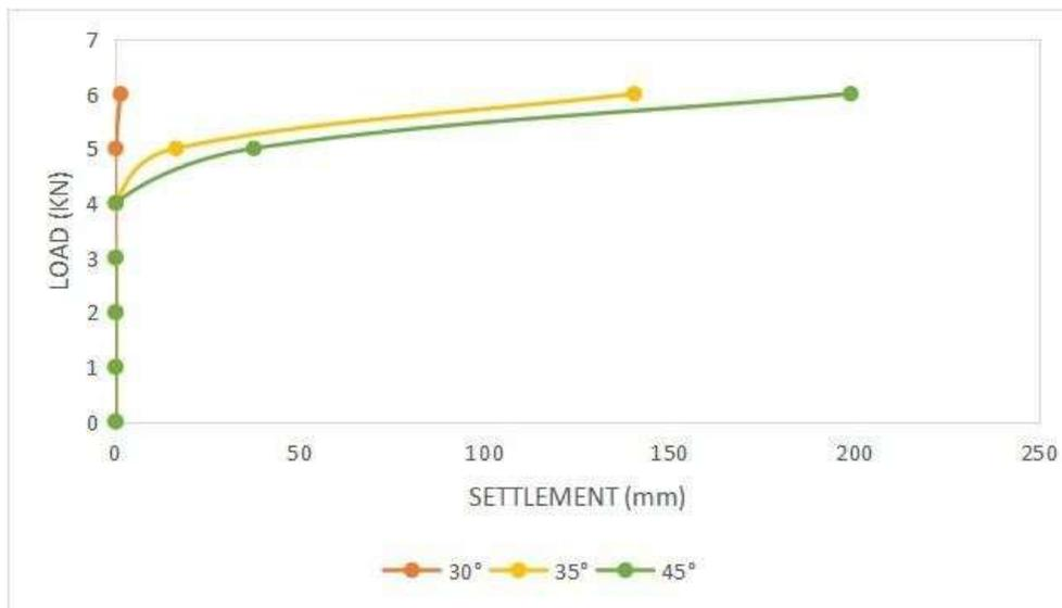
Fig. 3 Settlement Rate V/s Load graph for inclination of slope
