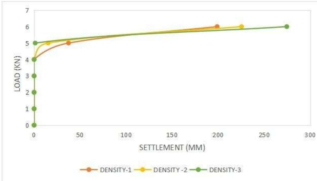
**Fig. 4** Settlement Rate V/s Load graph for Density of slope
