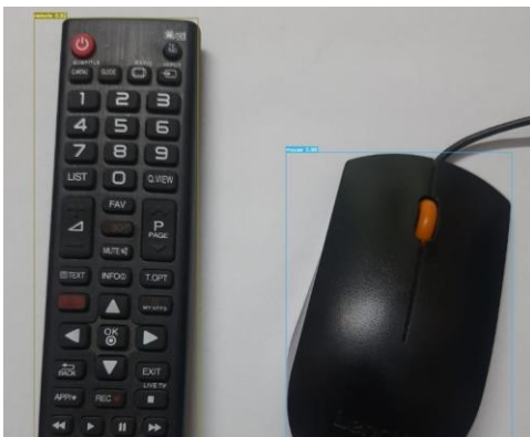
Fig. 8. A Remote and mouse are detected
