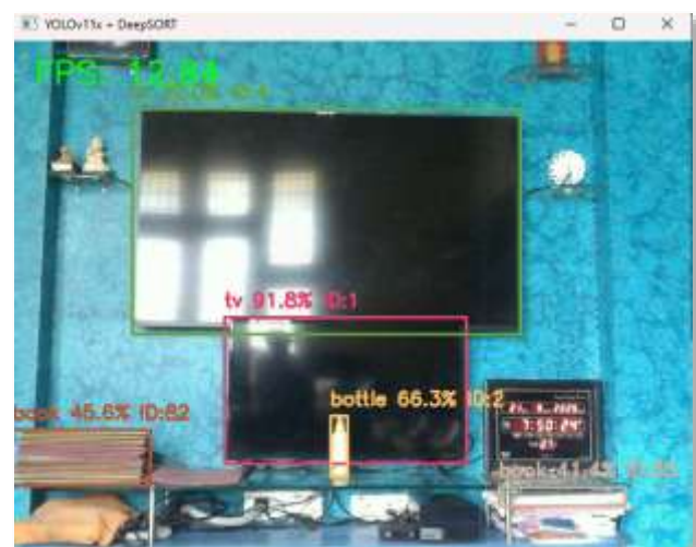
Fig. 6 Multiple Object Output of YOLOv11 and DeepSORT on Live Webcam Feed
