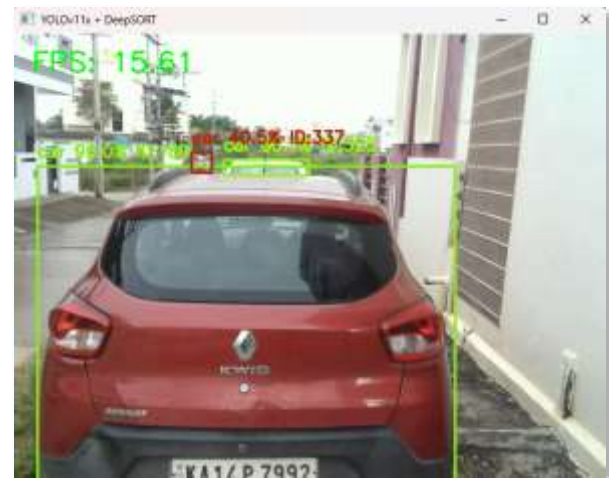
Fig 5. Result of Detecting Vehicle on the Road by Web Cam
