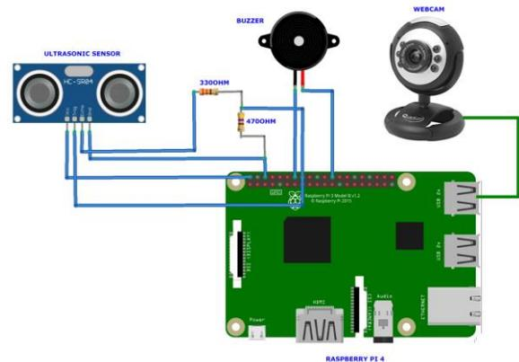
Fig -3: Circuit Diagram
