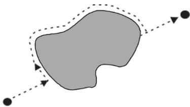
Fig -2: Demonstration of Bug Algorithm
