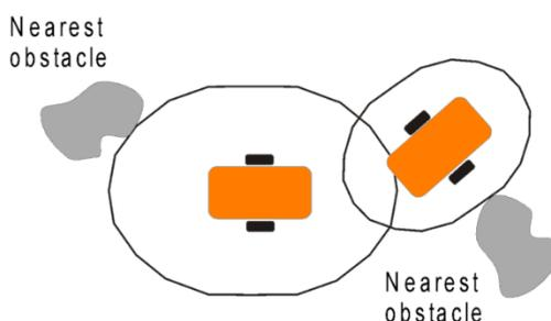
Fig -3: Demonstration of Bubble Band Technique
