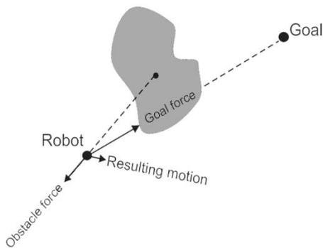
Fig -5: Demonstration of Potential Field Algorithm
