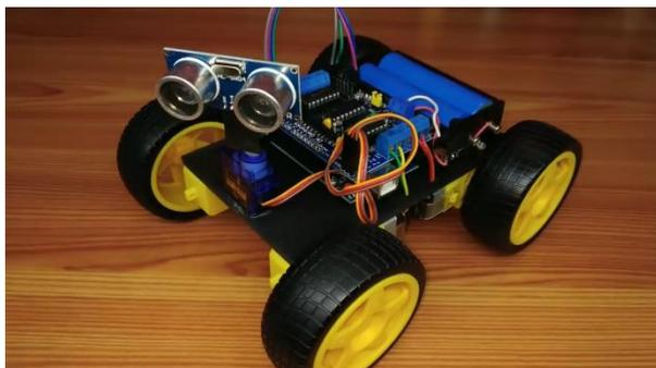
**Fig -8:** Working Model of Surveillance Robot
