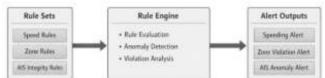
Fig. 4. Rule-based maritime monitoring framework used in Phase 2 of the proposed system.
