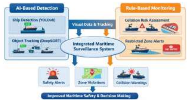
Fig. 1. Conceptual overview of the combined system showing AI-based detection and rule-based monitoring.
