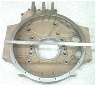
Fig -3: After machining part (frontview)
