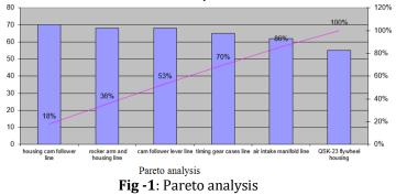
According to Pareto Analysis of all production lines of industry we came to conclusion that the OEE of QSK 23 housing flywheel line is less than all other production lines. So we set the target to increase its OEE by using lean manufacturing tools.
