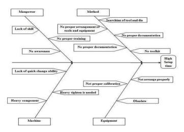
Fig -13: Fishbone diagram of high setup time of HMC machine
