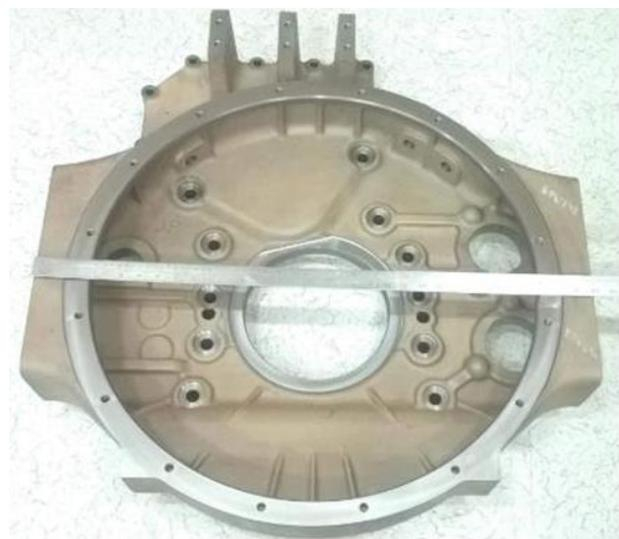
Fig -3: After machining part (frontview)
