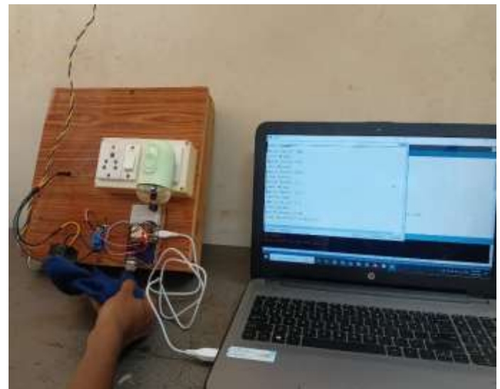
Figure 4: ESP32-Based Mouth Odor Detection System During Testing and Calibration
