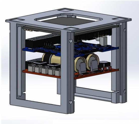
Figure 3. Slotted rack and dummy payloads
