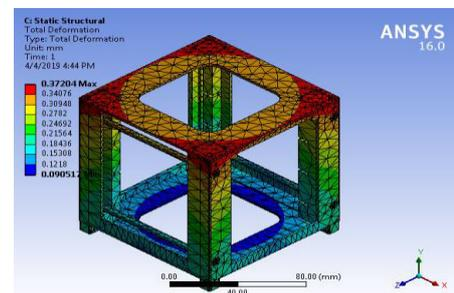
Figure 5(a). Total deformation
