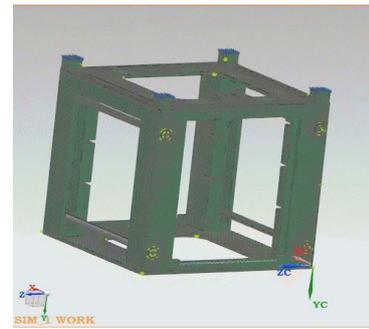
Figure 4. Fix Support in software analysis
