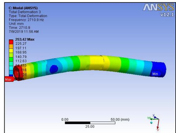
Fig.4.e (iii) Natural frequencies at 3rd node
