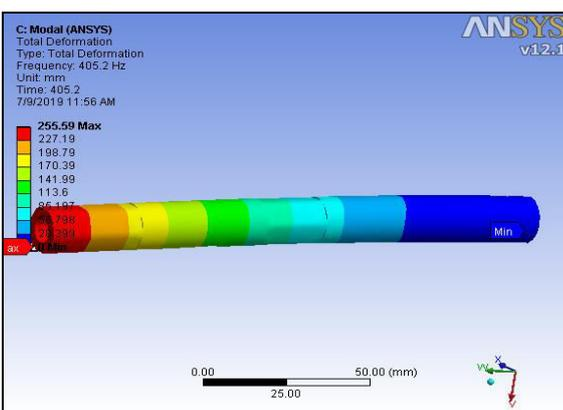
Fig.4.e (i) Natural frequencies at 1<sup>st</sup> node.
