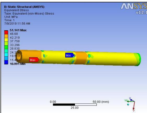
Fig.4.c Evaluating Equivalent Stresses
