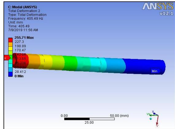
Fig.4.e (ii) Natural frequencies at 2<sup>nd</sup> node.
