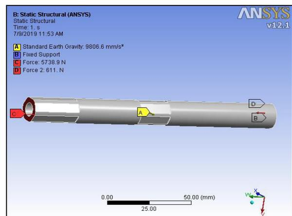
Fig.4.a Applying Boundary Conditions
