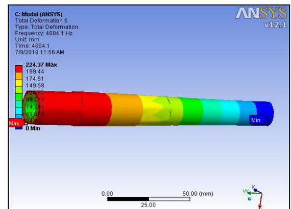
Fig.4.e (v) Natural frequencies at 5<sup>th</sup> node.
