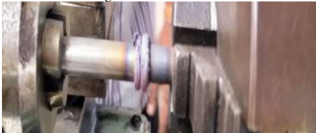
Fig - 3: welded joint
