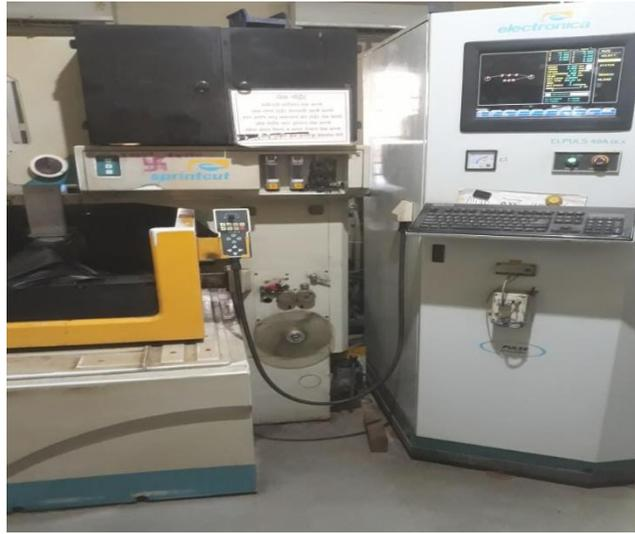
Figure.2.1 Setup Wire cut electro discharge Machine
