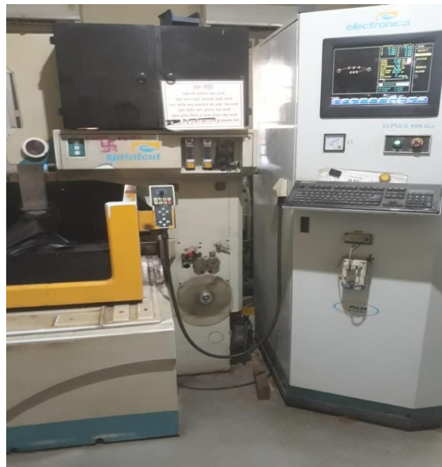
Figure.2.1 Setup Wire cut electro discharge Machine
