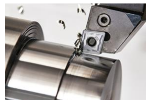
Fig. 1 : Dry Turning Process ( www.global-sei.com )
