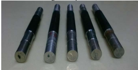
Fig 2: EN8 rods after machining operations
