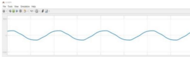
**Fig-4.** Final inverter output voltage waveforms The above graph is the final output of the voltage at the load, At the load, we can absorb the sinusoidal wave which means the AC supply
