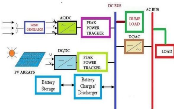
Fig-1. Block architecture of optimization of renewable energy for charging a battery.
