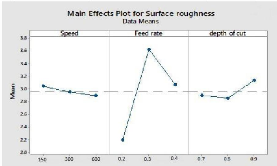
**Figure 4: Main effects plot for means for surface roughness for wet turning**
