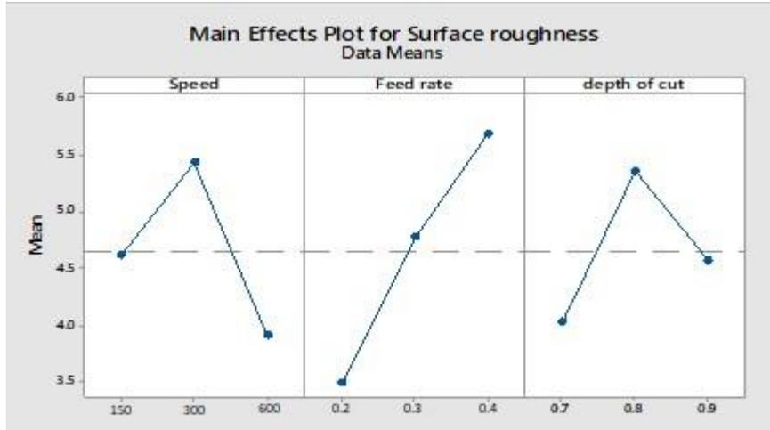
**Figure 3: Main effects plot for means for surface roughness for dry turning**
