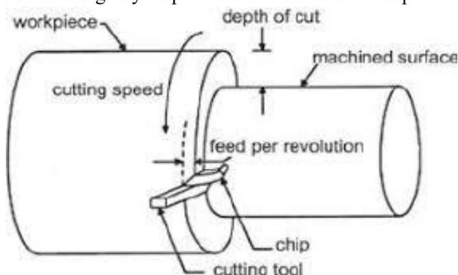
Figure 1: Turning Process
