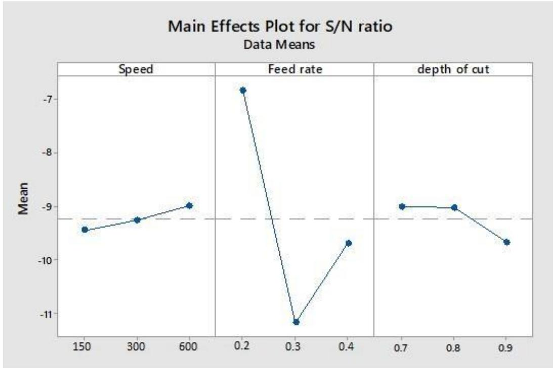
Figure 6: Main effects plot for S/N ratios for surface roughness in Wet Turning
