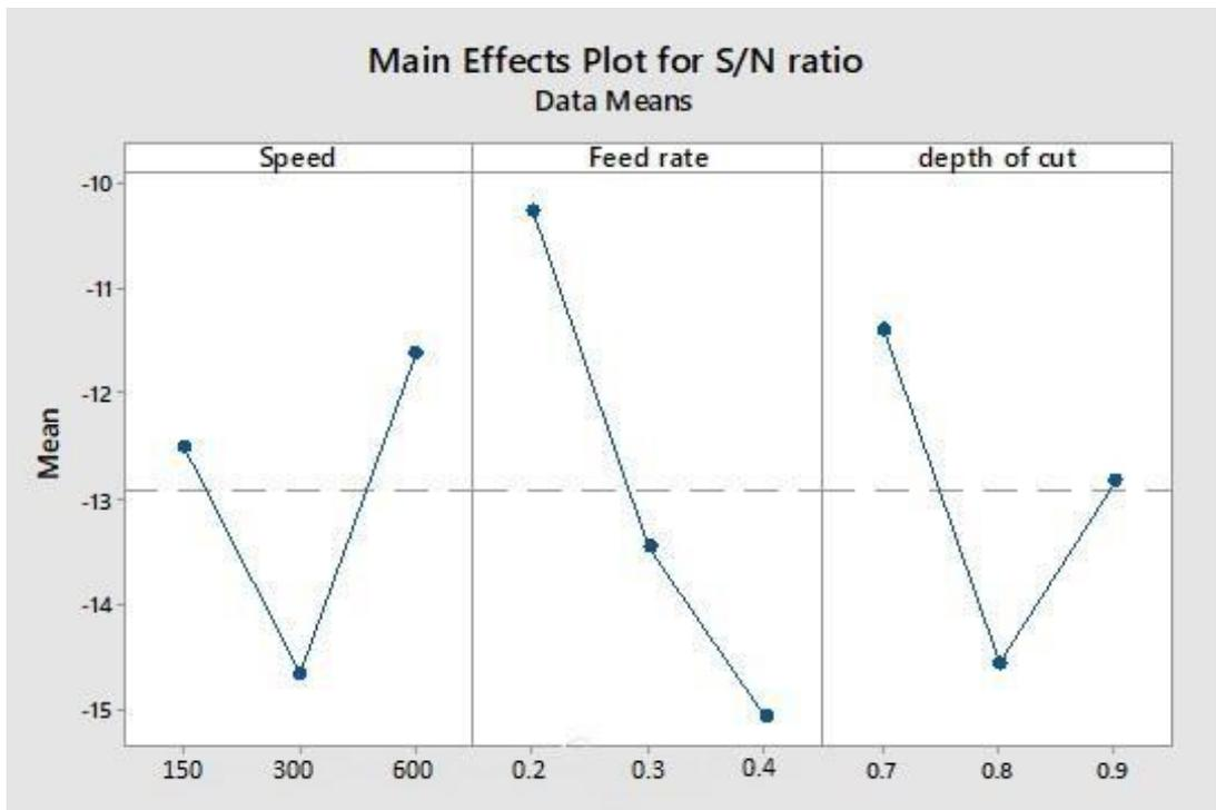
**Figure 5: Main effects plot for S/N ratios for surface roughness in Dry Turning**
