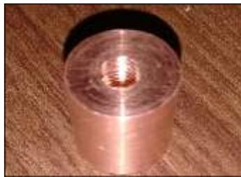
Fig 1. Copper tool of 10mm diameter
