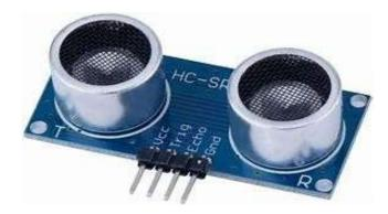
Fig3.Ultrasonicsensor DCGear Motor
