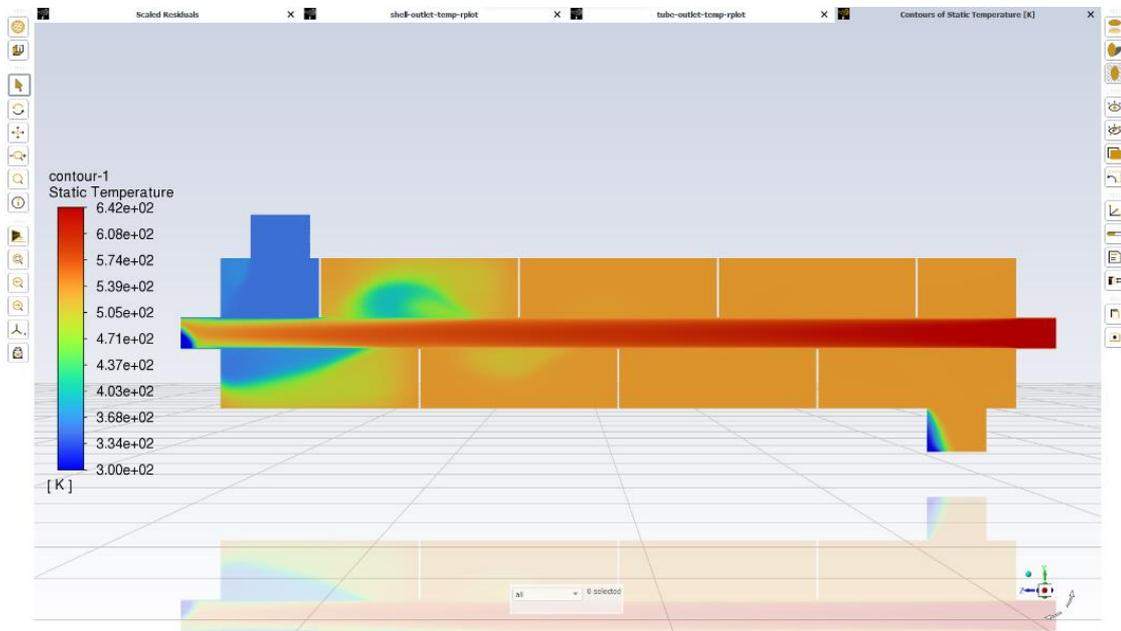
Fig. 3 Contour of static temperature of model A in a mid-plane
