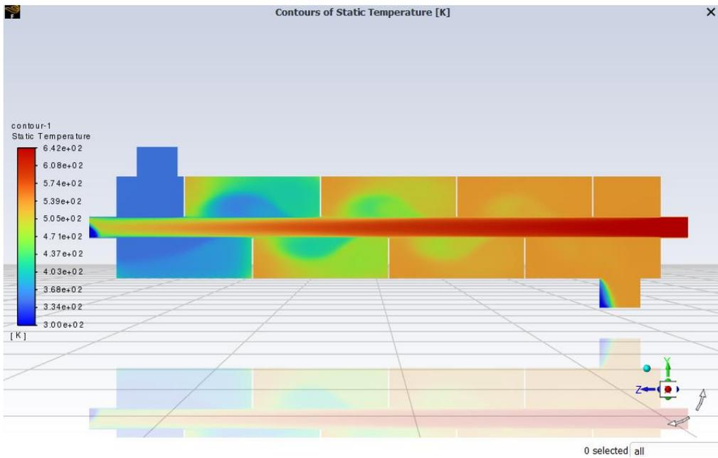
Fig. 6 Contour of static temperature of model B in a mid-plane
