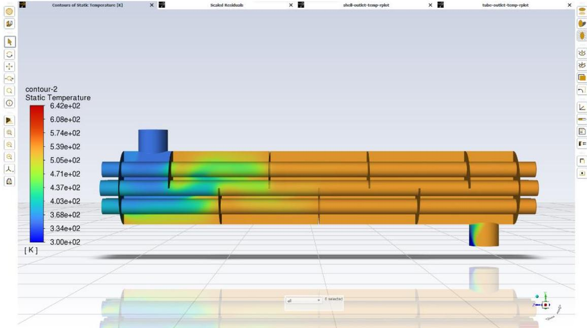
Fig. 2 Contour of static temperature of model A
