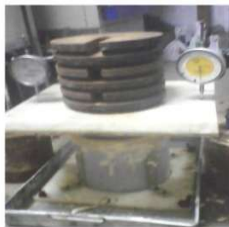
Figure2: Applying 2nd load @0.11kg/sq.cm
