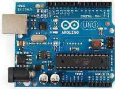
Fig. 2: Arduino Uno Microcontroller Development Board
