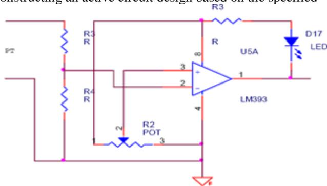
Fig -2: Circuit diagram of overvoltage protection
