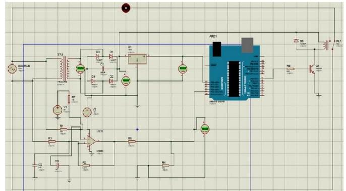
Fig -3: Design of under voltage and over voltage control system using Proteus software
