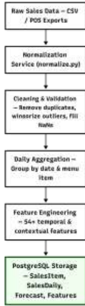
Fig. 2: Data preprocessing flow including normalization, validation, cleaning, aggregation, and feature extraction for each item-day record.
