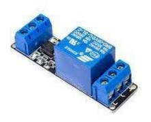
A relay is an electrically operated switch. It consists of a set of input terminals for single or multiple control signals and a set of operating contact terminals. The switch may have any number of contacts in multiple contact forms, such as make contacts, break contacts, or combinations thereof. Relays are used where it is necessary to control a circuit by an independent low-power signal, or where several circuits must be controlled by one signal.
