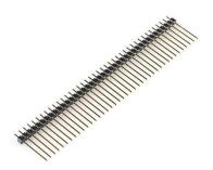
Pin headers are stiff metallic connectors that are soldered to a circuit board and stick up to receive a connection from a female socket. While pin headers (often called PH, or headers) are male by definition, female equivalents are also quite common, and we refer to them as female headers (FH) or header connectors.
