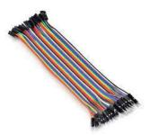
Jumper wires are simply wires that have connector pins at each end, allowing them to be used to connect two points without soldering. Jumper wires are typically used with breadboards and other prototyping tools to make it easy to change a circuit as needed.
