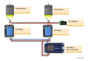
NodeMCU is an open-source IoT platform. It includes firmware that runs on the ESP8266 Wi-Fi SoC from Espressif Systems, and hardware that is based on the ESP-12 module. The term "NodeMCU" by default refers to the firmware rather than the development kits. The firmware uses the Lua scripting language. It is based on the eLua project, and built on the Espressif Non-OS SDK for ESP8266. It uses many open-source projects, such as lua-Jason and SPIFFS.
