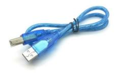
USB stands for Universal Serial Bus. It is used as a data cable for programming as well as for supplying power.
