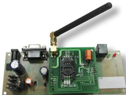
Fig-4: GSM Module
