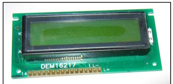
Fig-2: LCD Display Module
