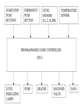
The given block diagram represents the control system of an automated boiler project using a Programmable Logic Controller (PLC). The system is designed to manage the water level, temperature, and various actuators involved in the boiler operation. The major components are described below:
