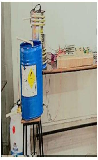
The system has been successfully designed and implemented for the automation of a water tank, with continuous monitoring and measurement of parameters such as temperature and level. The entire reactor water tank process is managed by a Programmable Logic Controller (PLC), which converts analog signals into the necessary digital format. Real-time temperature and level data are visually represented in the SCADA system through graphical displays.
