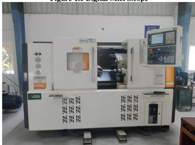
Figure:3.2 Ace Microsmatic SJ 500 XL CNC Lathe Machine, Length: 500 mm
