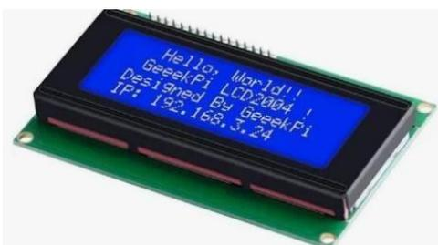
LCDs are frequently employed in portable electronic games, as viewfinders for digital cameras and camcorders, in video projection systems, for electronic billboards, as monitors for computers, and in flat-panel televisions. In our project, we developed a smart parking system that utilizes an LCD display to provide real-time information about parking spaces, including the number of available spots and the number that are currently occupied.
