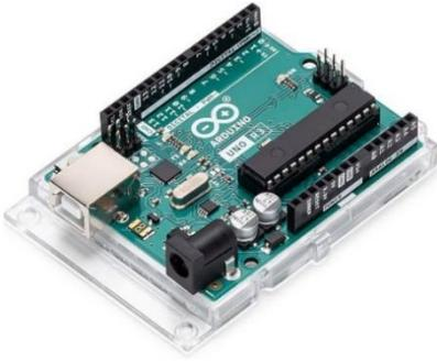
The Arduino Uno serves as the primary component of this project, acting bridge between the software and hardware aspects. The physical component of the undertaking. Arduino board is a kind of microcontroller. It receives data from sensors, regulates the servo motor, interacts with the wifi module, and operates the lcd display
