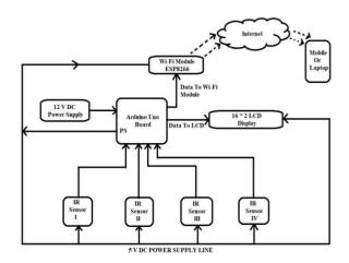
• Vehicle detection: infrared sensors are installed at exit and entry point and parking spaces to detect vehicles. When a car enters, the sensor recognizes the space as occupied, while a free slot is detected when car is not present.
