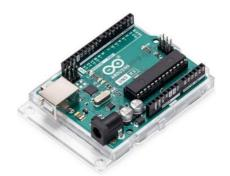
The Arduino Uno serves as the primary component of this project, acting bridge between the software and hardware aspects. The physical component of the undertaking. Arduino board is a kind of microcontroller. It receives data from sensors, regulates the servo motor, interacts with the wifi module, and operates the lcd display
