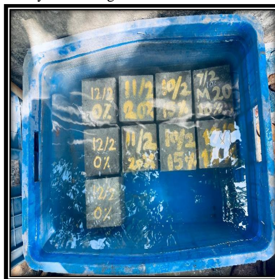
Fig-3: Concrete Cube Curing
