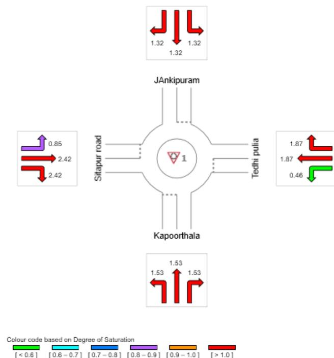
Figure 4 Degree of Saturation for 4-legged roundabout
