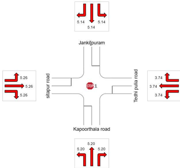
Figure 3 Degree of saturation for 4-legged intersection
