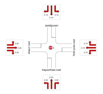
Figure 3 Degree of saturation for 4-legged intersection
