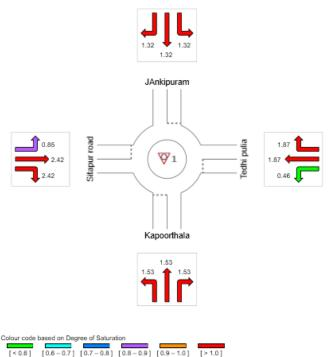
Figure 4 Degree of Saturation for 4-legged roundabout
