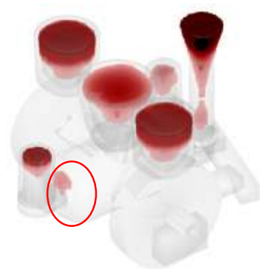
FIGURE 5. Defect after Solidification
