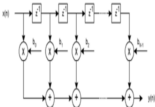
Figure 1.2: Basic structure of FIR filter.
