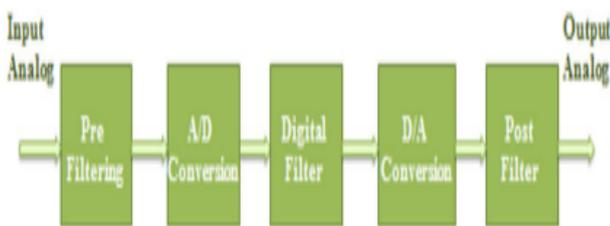
Figure 1.1: Block diagram of digital filtering process.
