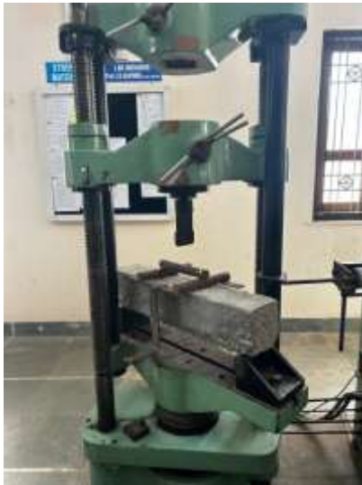
Fig. 4: Flexural Strength Testing
