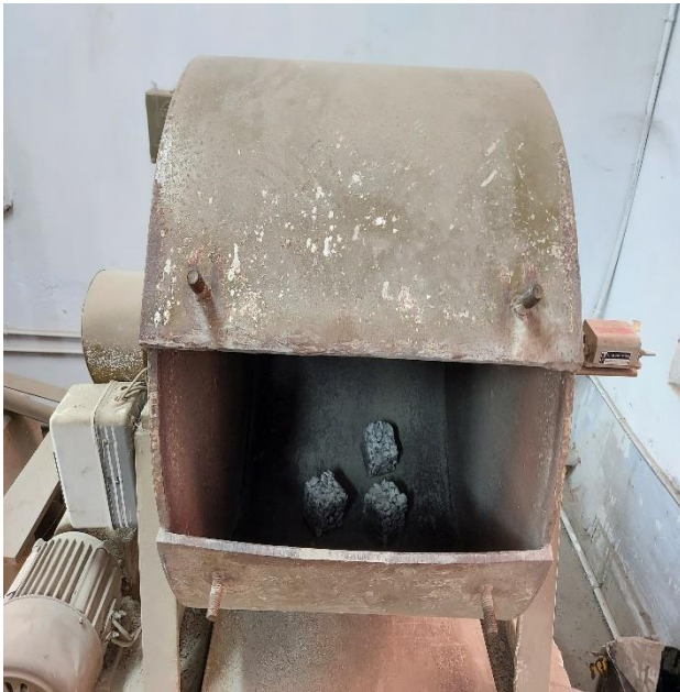
Fig.3.8 Los Angeles Abrasion Machine
