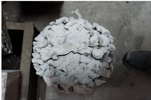
Fig. 4.2 Failure of split tensile strength
