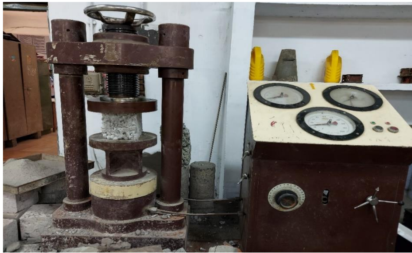
Fig 3.3 Compressive strength on trial mix specimen
