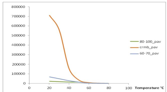
Fig.8. Complex Modulus versus temperature
