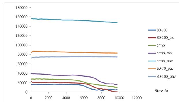
Fig.4 Complex shear modulus  $G^*$  versus stress
