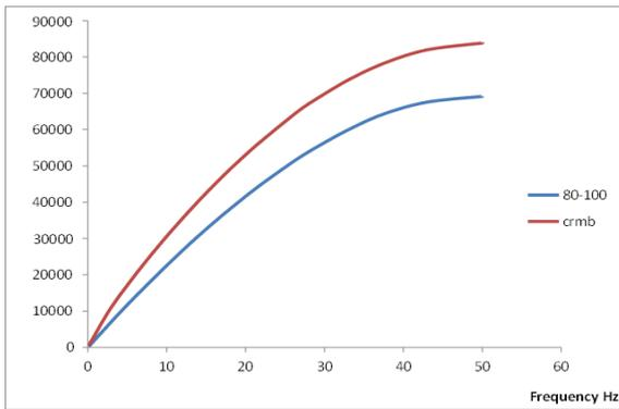
Fig.5. Complex modulus versus frequency for neat bitumen
