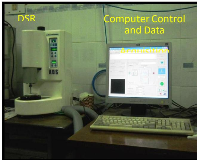
Fig.1 Dynamic Shear Rheometer
