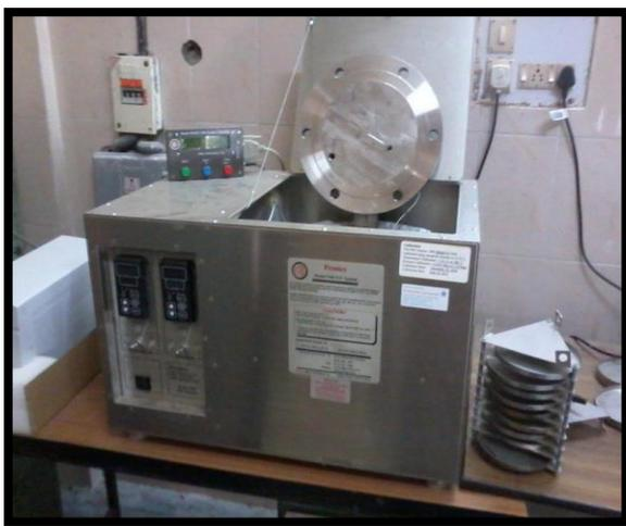
Fig.3 Pressure Vessel Ageing for long term ageing
