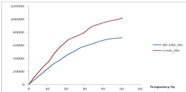
Fig.6 Complex modulus versus frequency for short term aged bitumen
