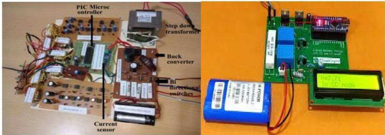
Fig 9; Blocks in the hardware prototype.
