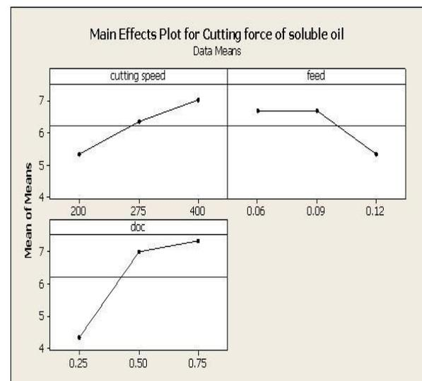
**Fig.2** –Main effects plot for cutting force of soluble oil
