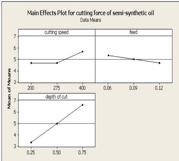
Fig.3 –Main effects plot for cutting force of semi-synthetic oil
