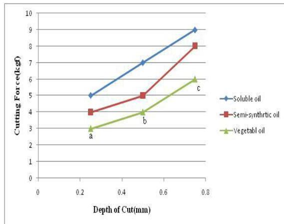
**Fig.8-** Depth of cut Vs. Cutting force, cutting speed: 400rpm; feed: 0.09, 0.12, 0.06mm/rev at the three points a, b and c, respectively.
