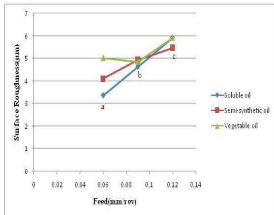
**Fig.9-** Feed Vs. Surface Roughness, cutting speed: 400rpm; depth of cut: 0.75, 0.25, 0.50mm at the three points a, b and c, respectively.
