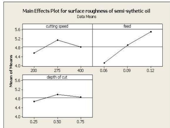
Fig.6 –Main effects plot for surface roughness of semi-synthetic oil
