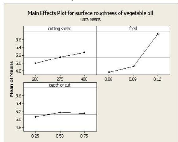
Fig.7 –Main effects plot for surface roughness of vegetable oil
