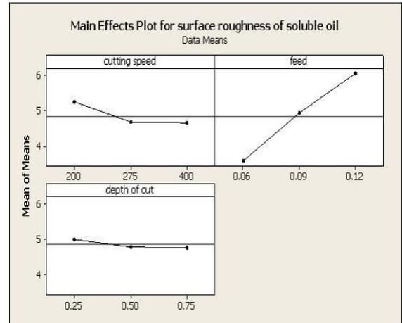
Fig.5 –Main effects plot for surface roughness of soluble oil
