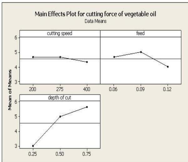
Fig.4 –Main effects plot for cutting force of vegetable oil
