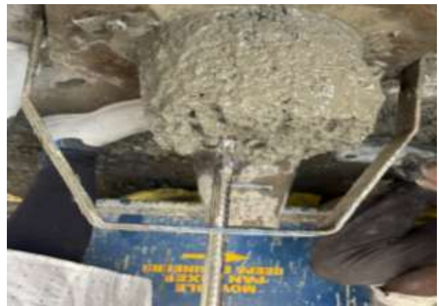
Fig 6: Slump test of the fresh concrete mix.
