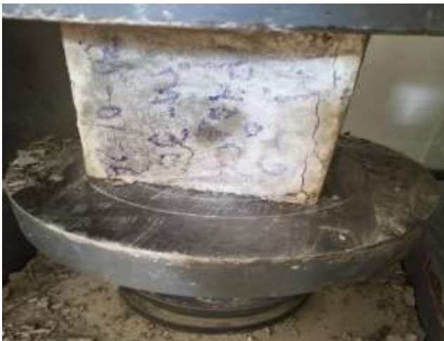
Fig 8: Concrete specimen showing failure patterns under axial loading.
