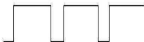
Fig 4. Mark space ratio (75% duty cycle)
