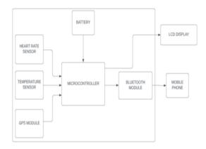
The primary power source of the system is a battery, which supplies energy to an Arduino Uno microcontroller board. The Arduino Uno acts as the central processing unit, responsible for coordinating the operation of the entire system. Connected to the Arduino Uno are three essential input components:
